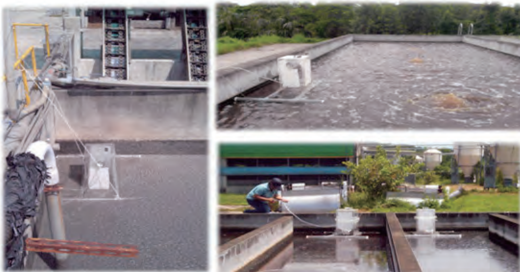
Methane emission collected by sampling hood
