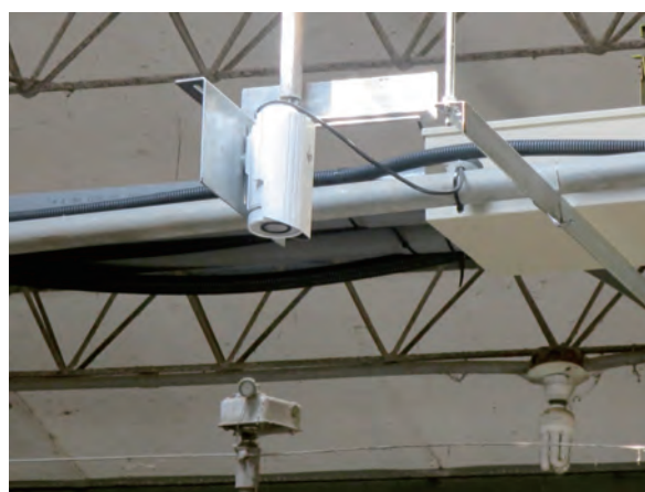
The equipment of imaging monitor of laying cage of RFID in breed geese
