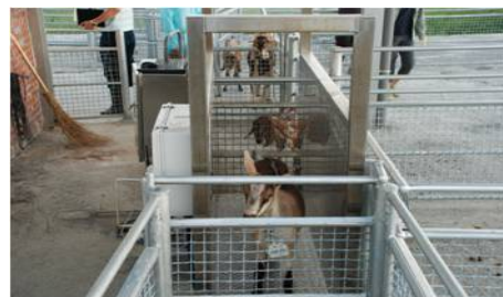
Electronical goat handling system that combines ultrahigh RFID electronic ear tags with auto-weighing scale
