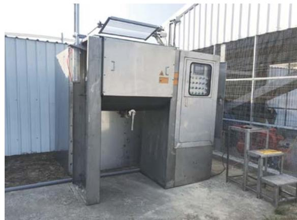
Prototype of small scale high biosafety poultry manure processing system
