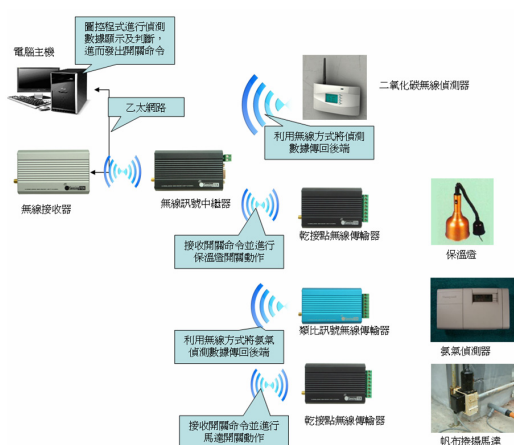
▲無線感測網路(Wireless sensor network, WSN)應用於生醫用小型豬畜舍之圖示
