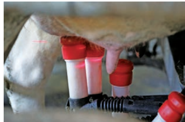
The design of separated-operation cups in the auto-milking system contributes to the reduction of teat injuries
