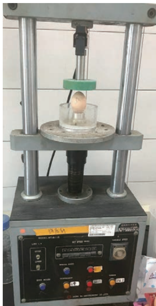
Egg shell breaking strength-meter
