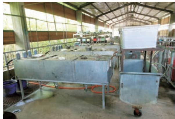
Pig wastewater treatment module
