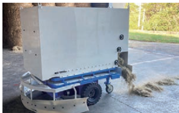
The prototype machine of automatic feeding developed by domestic institutions for dairy cows
