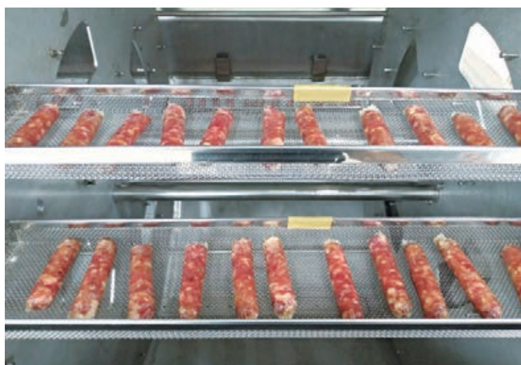
The sausages drying process in vacuum (a) and microwave (b) chambers
